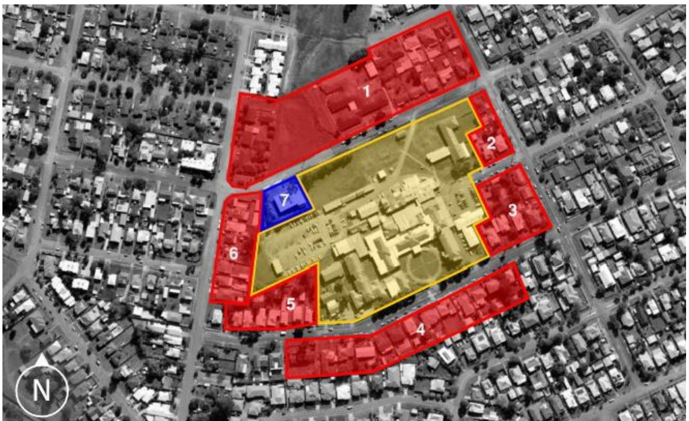
Figure 14 Nearest noise sensitive receivers surrounding the site
